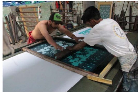
Figure-4. Manual process of screen printing in SMEs.
